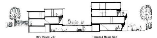
4. Section through street at Row House Unit, left and one type of Terraced House Unit, right. 6-8 Vendome Place uses both layouts though some buildings have sloped roofs (Grossman 1961:64).
