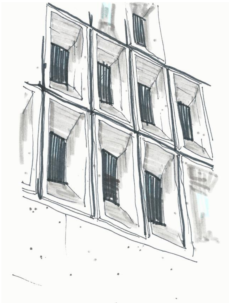
Sketch of the façade of concrete units
